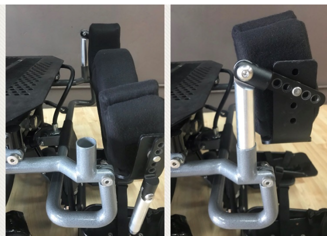
Figure 26 - Left: removed knee bolster. Right: fully inserted knee bolster pin.
